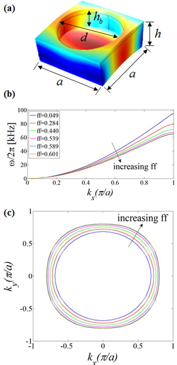
FIG. 1. (a) Schematic of the square unit cell structure of the GRIN-PCL plate with blind holes. (b) Band structure of the  $A_0$  mode for various filling factors ( $ff = \pi d^2/4a^2$ ). (c) Equal frequency contours of the  $A_0$  mode Lamb wave at 50 kHz.
